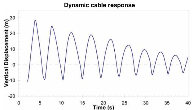
Fig.2a Vertical displacement at the mid-span point, following sudden shedding on the entire span
