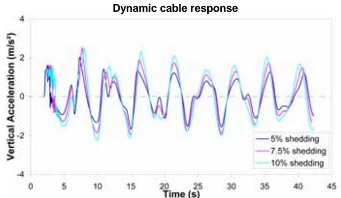
Fig.4c Vertical acceleration of the node adjacent to the last snow-shedding element, following partial shedding at 14 m/s
