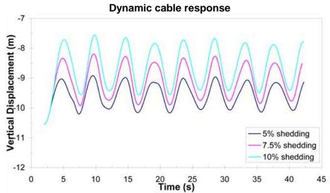
Fig.4a Vertical displacement at the mid-span point, following partial shedding at 14 m/s
