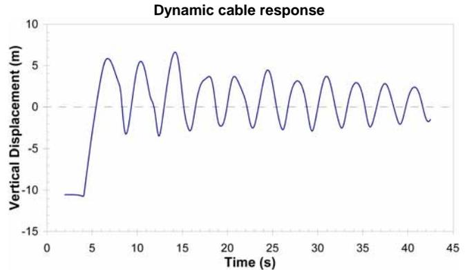
Fig.3a Vertical displacement at the mid-span point, following total shedding at 111m/s
