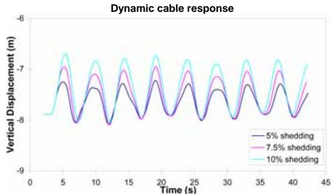
Fig.4b Vertical displacement at the quarter-span point, following partial shedding at 14 m/s
