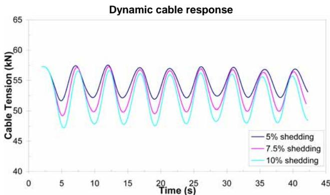
Fig.4e Cable tension at the end point, following partial shedding at 14 m/s
