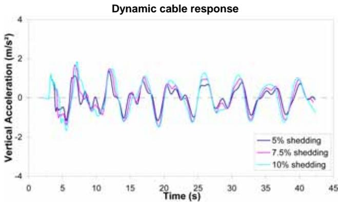
Fig.4d Vertical acceleration at the quarter-span point, following partial shedding at 14 m/s
