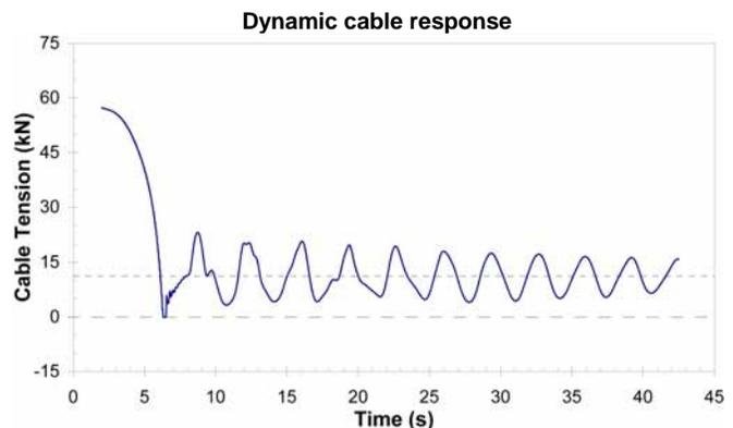
Fig.3c Cable tension at the end point, following total shedding at 111m/s
