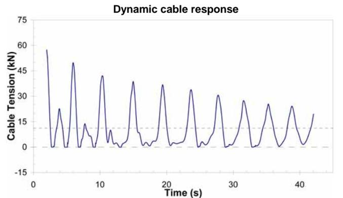
Fig.2b Cable tension at one end, following sudden shedding on the entire span
