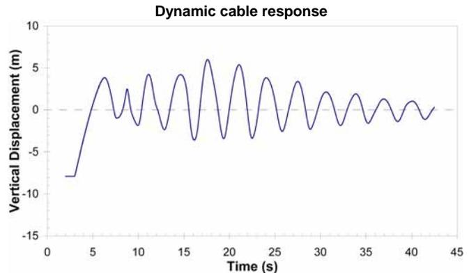
Fig.3b Vertical displacement at the first quarter-span point, following total shedding at 111m/s
